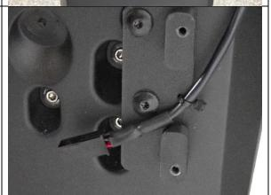
Connect the ID light set to the cable and secure with the four black screws provided in the kit.
