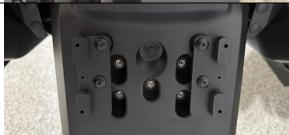
Position the pre-assembled License Plate ID Light Set onto the License Plate Mount Set to determine location of the cable exit point. Cable tie the cable to the RH license plate mount as shown at right.
